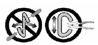
Notice: It is important to use proper chain pliers (not included) To OPEN and CLOSE the chain included with this fixture. Do not open them with other tools that may twist or stress the chain links. It is important to use proper chain pliers like the ones shown in the diagram.
