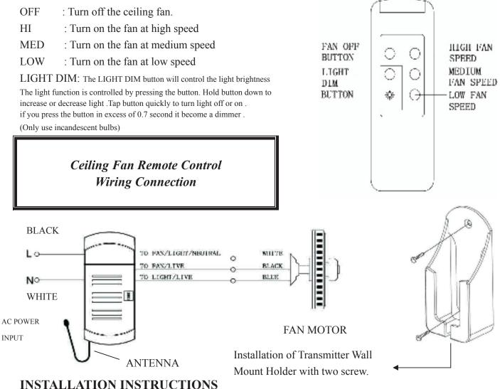
CAUTION: INCORRECT WIRE CONNECTION WOULD DAMAGE THIS RECEIVER.
